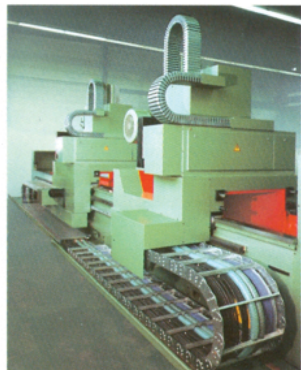
6 Combined production machine with milling and grinding carriage. CNC controlled, 6 axes
