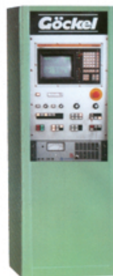
Control desk with screen CNC-multifunction key- board integrated machine control board and electro- nic handwheel
