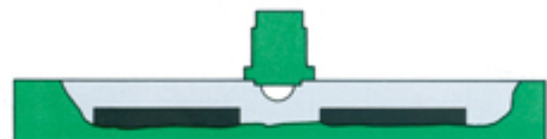
One grinding head carriage two-stationary grinding e.g. clamping to the left, grinding to the right
